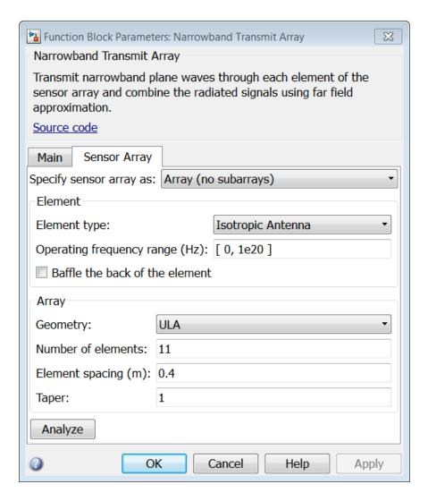
Click Analyze to open the Sensor Array Analyzer app and show the array directivity.
